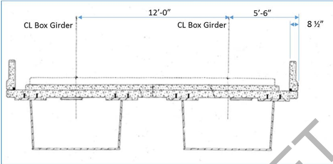
FIGURE 5: CROSS SECTION OF BOX GIRDERS
