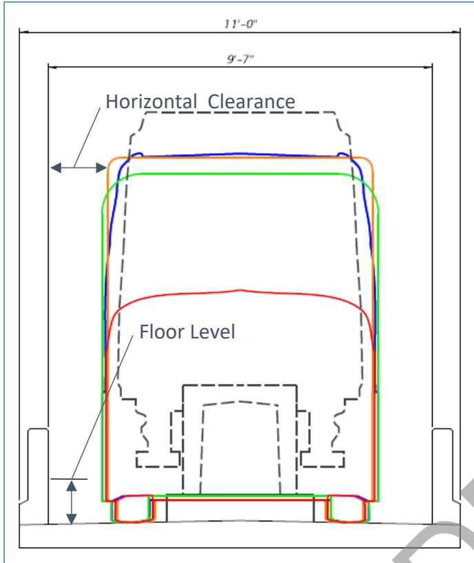
FIGURE 18: HORIZONTAL CLEARANCE
