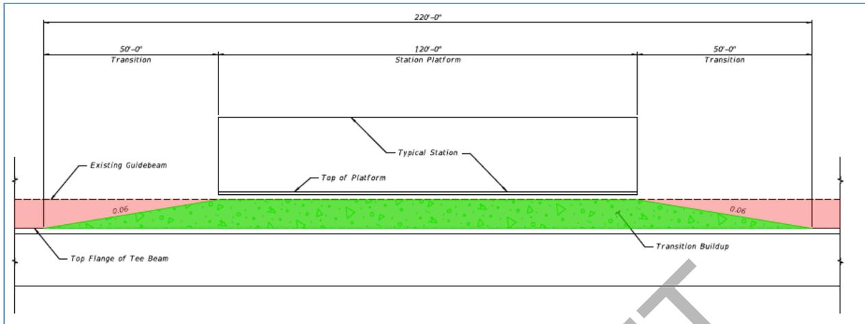
FIGURE 34: ELEVATION VIEW OF PLATFORM
