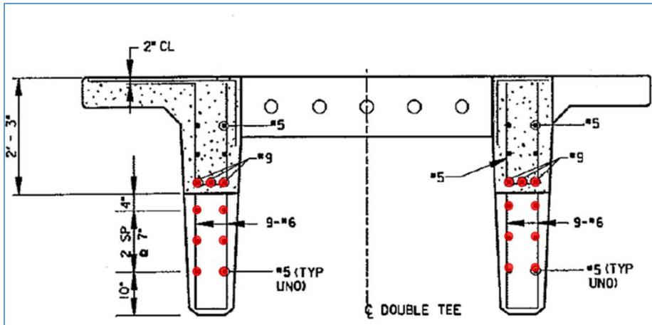
FIGURE 37: FIXED BEAM (END VIEW)
