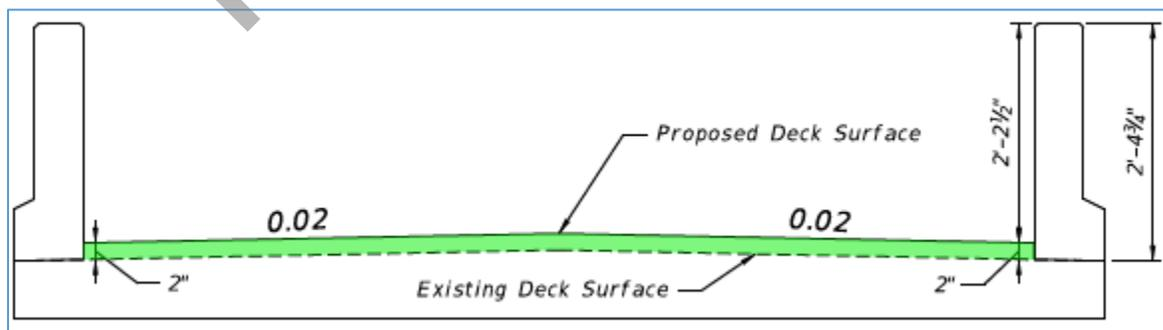
FIGURE 26: NORMAL CROWN TYPICAL SECTION WITH OVERLAY
