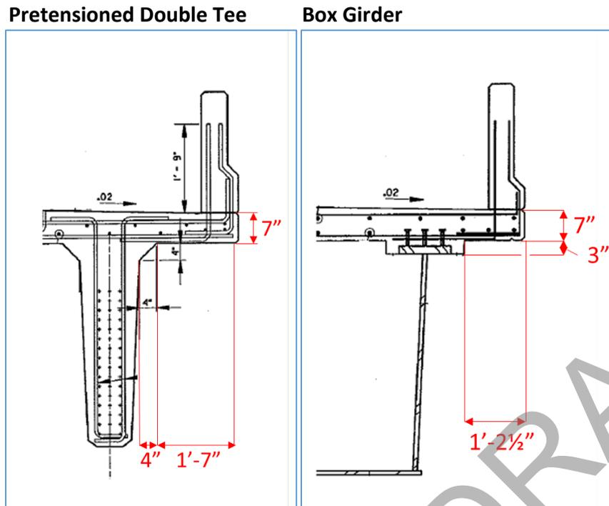
FIGURE 23: DECK SECTION DETAILS (SOUTH LINE AS-BUILTS)
