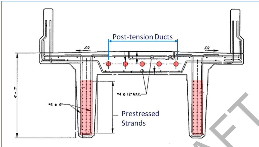
FIGURE 7: PRESTRESSED AND POST-TENSIONED DETAIL
